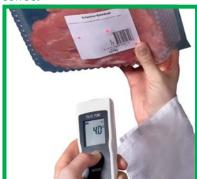
The diameter of the entire measurement spot must always be on the measured item
